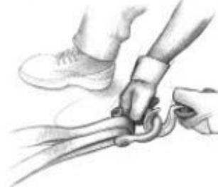
**D-ring shackle** is a great tool, but it's heavy and thus stores lots of potential energy when under load. If it fails, it will travel fast with plenty of force to kill you. Be sure it is oriented correctly and the pin is screwed in tight, then back off  $\frac{1}{2}$  turn.
