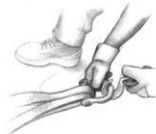
**D-ring shackle** is a great tool, but it's heavy and thus stores lots of potential energy when under load. If it fails, it will travel fast with plenty of force to kill you. Be sure it is oriented correctly and the pin is screwed in tight, then back off ½ turn.
