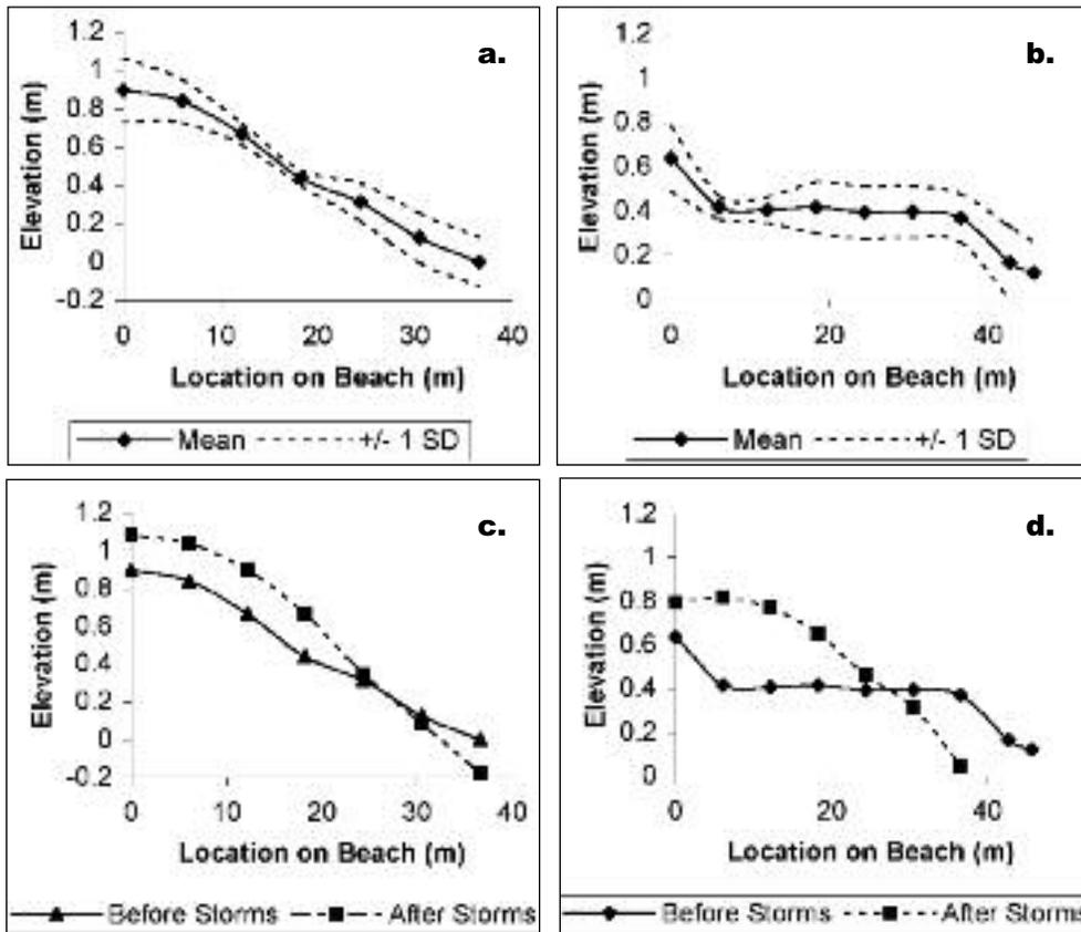
Figure 9. Sand accretion on the Miramar experimental site and the adjacent control site between May and October 2002: (a) experimental site, May 2002; (b) control site, May 2002; (c) experimental site, May and October 2002; (d) control site, May and October 2002.
