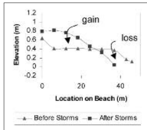
Figure 10. Sand gain and loss based on profile measurements.
