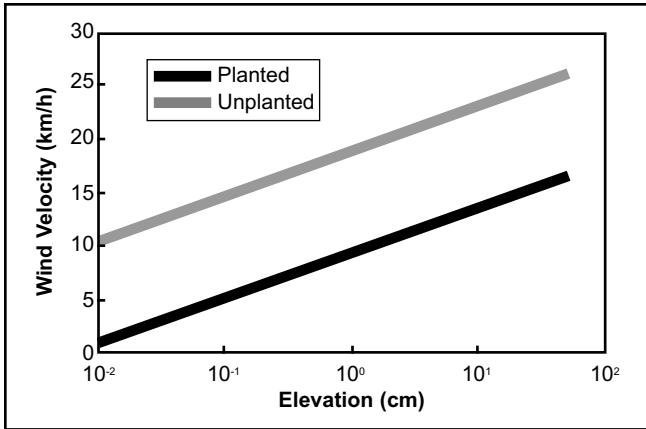
Figure 11. Semi log plot of predicted wind velocity above the sand surface.
