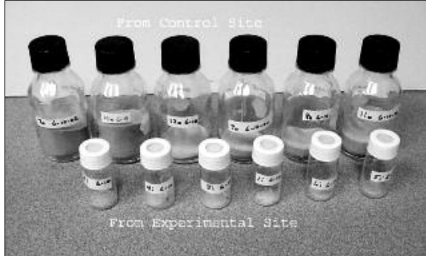
Figure 13. Sand captured in Leatherman tubes on the experimental site (small bottles) and on the control site (large bottles) over a 15-hour period.
