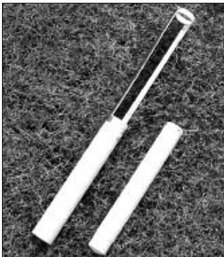
Figure 12. Leatherman tubes used to measure wind transport of sand on the beach.
