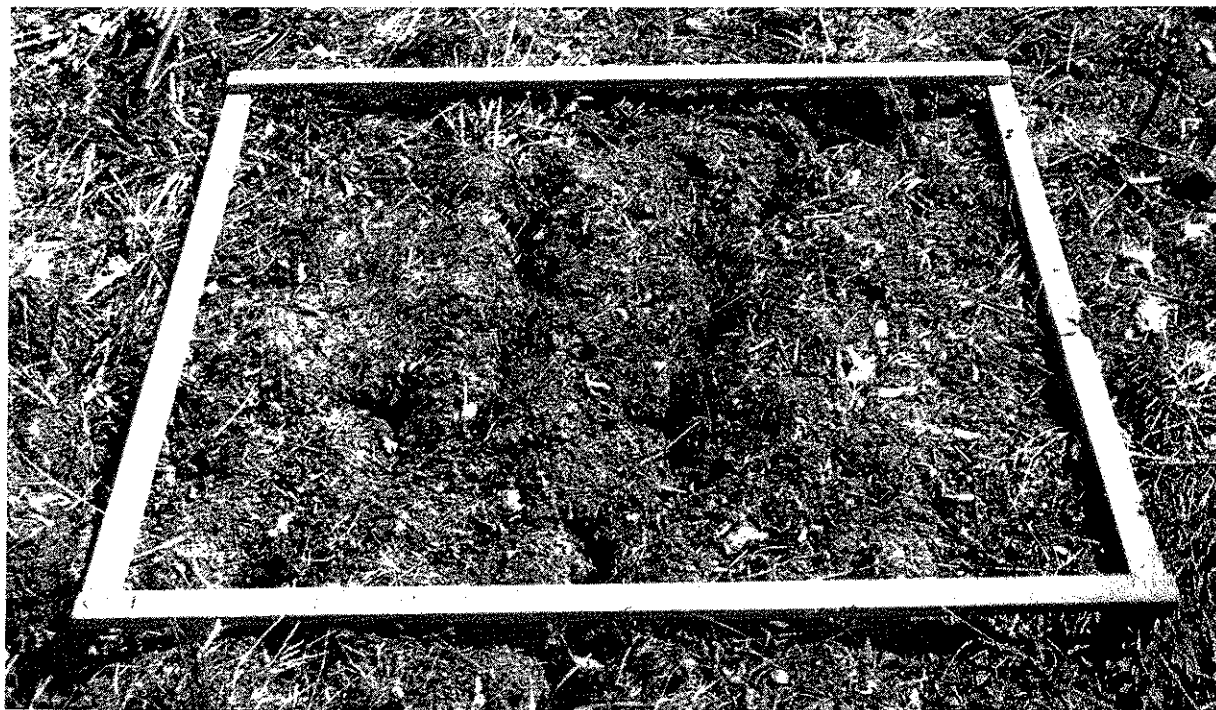
Figure 2. Surface crack research plot (11 ft 2 ) in an Alligator clay soil in Leflore County.
